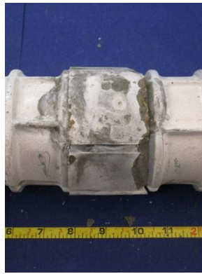
Figure 5.66: Specimen 3.1, Cement Paste and Large Aggregate Embedded in North Grout
