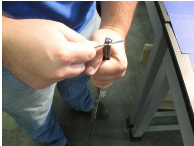
Figure 5.10: Using Screwdriver to Unravel Strand
