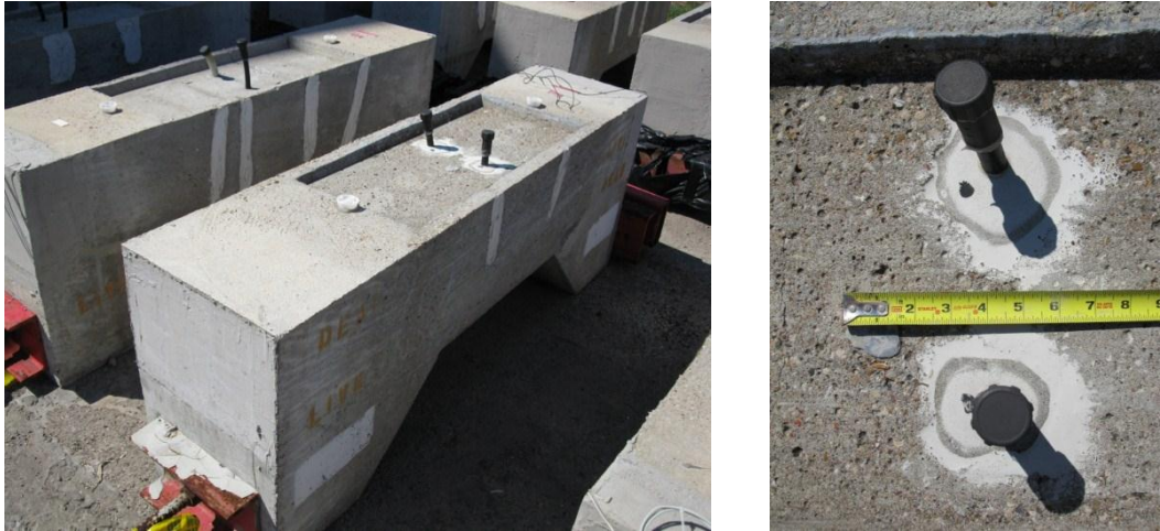
Figure 5.22: Specimen T.2 Overall (Left) and Grout Vents (Right)
