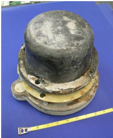
Figure 5.112: Specimen 7.1 Anchorage Components, from Top: Grout Cap, Retaining Ring, Insulation Plate, Bearing Plate
