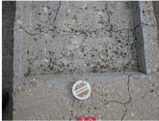
Figure 5.75: Specimen 3.2, Black Residue in Saltwater Tray
