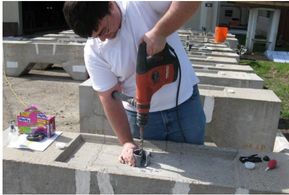
Figure 3.8: Chloride Sample Extraction with Hammer Drill
