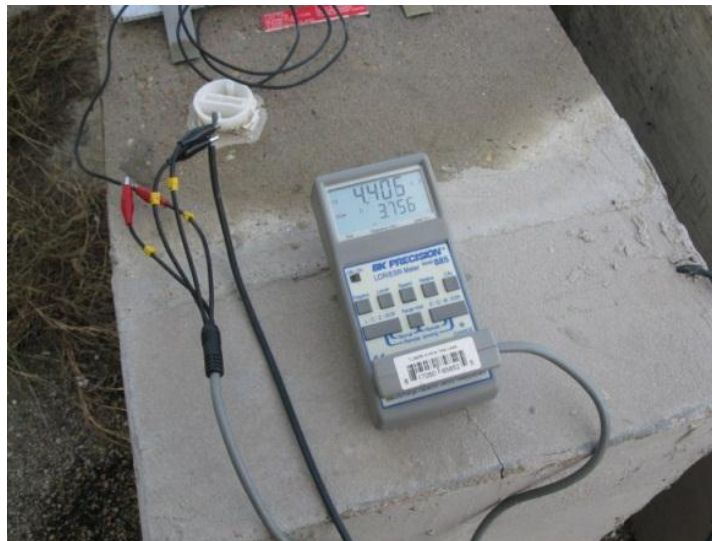
Figure 3.6: LCR Meter Connected to Specimen to Measure AC Impedance
