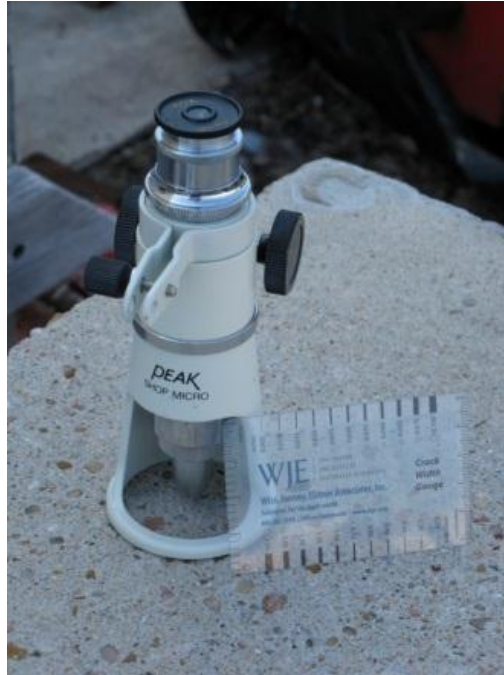
Figure 5.1: Crack Width Measurement Tools
