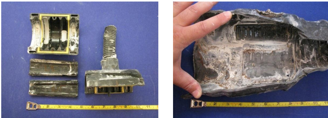
Figure 5.109: Specimen 7.1 Live End Coupler (Left) and Live End Sheath (Right)
