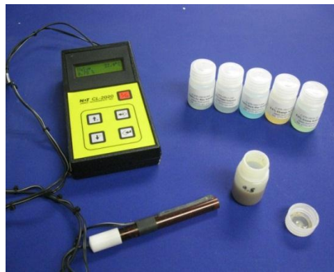
Figure 3.7: Chloride Content Measurement Setup
