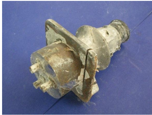
Figure 5.8: Dead End Anchorage from Specimen 4.2 Showing Saw Damage
