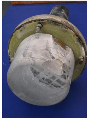
Figure 5.114: Specimen 7.1 Dead End Grout Cap Showing Grout Discontinuity
