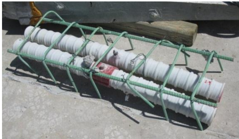
Figure 5.7: Reinforcement Cage and Post-Tensioning Tendons from Specimen 2.4
