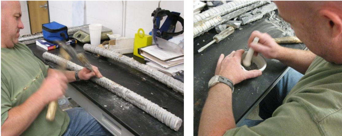
Figure 3.11: Grout Chloride Sample Extraction (Left) and Grinding (Right)
