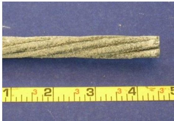
Figure 5.78: Specimen 3.2, Bubbles in Interstices of Galvanized Strand
