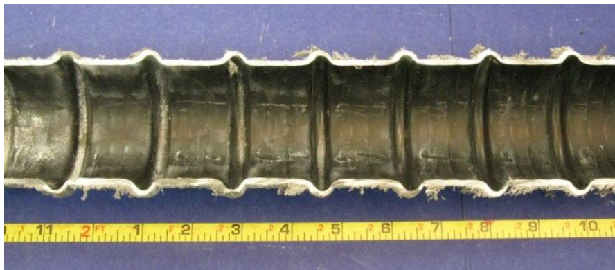
Figure 5.89: Specimen 3.4, Strand Gouging on Bottom of North Duct
