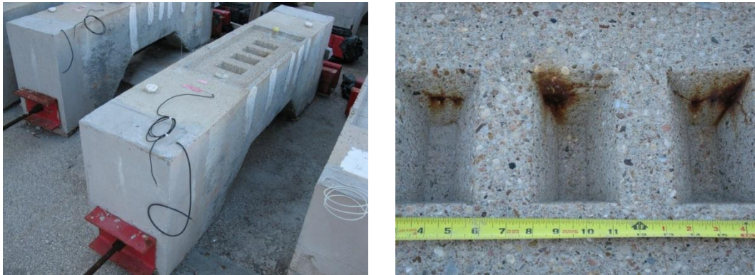
Figure 5.106: Specimen 7.1 Overall (Left) and Corrosion Staining in Saltwater Tray Wells (Right)
