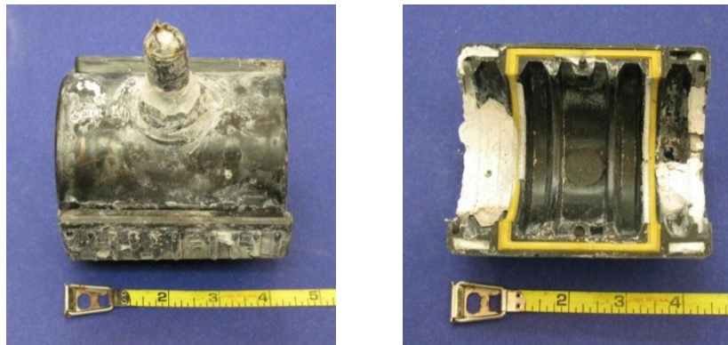
Figure 5.99: Specimen 4.2 Coupler Outer Surface (Left) and Lower Gasket Breach (Right)
